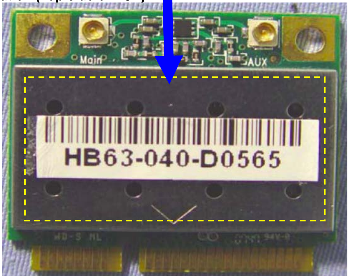
Label location (Top side of EUT)
