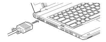
Figure 42. Connecting an External Video Device
