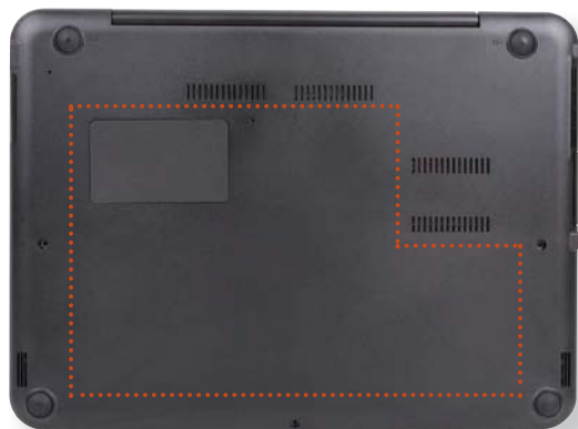
The location of the internal battery
