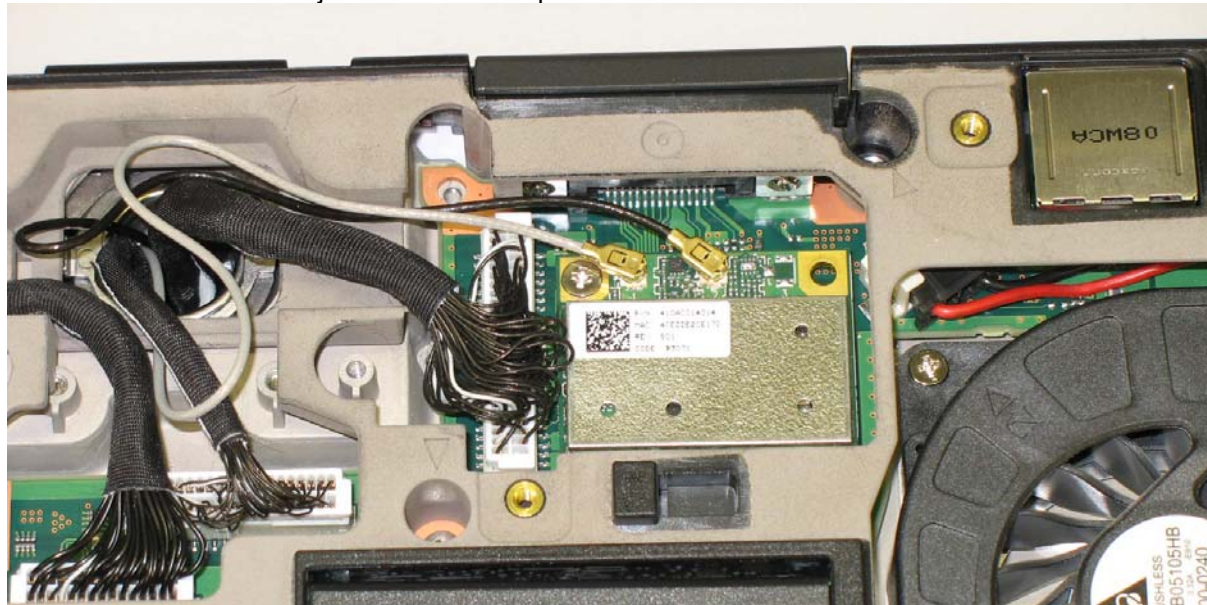
AR5BHB116 inside the Fujitsu TABLET Computer
