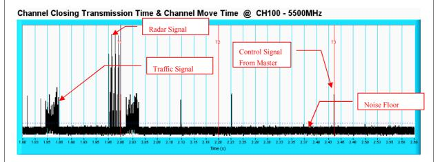
**NOTE:** An expanded plot for the device vacates the channel in the required 200ms.
