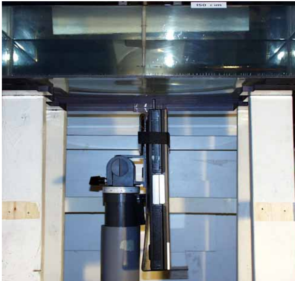
< Edge of the card pointed toward the phantom, 15 mm separation distance, Prescan >
