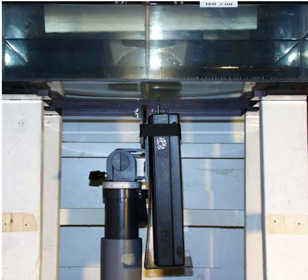
< Edge of the card pointed toward the phantom, 15 mm separation distance, Prescan >
