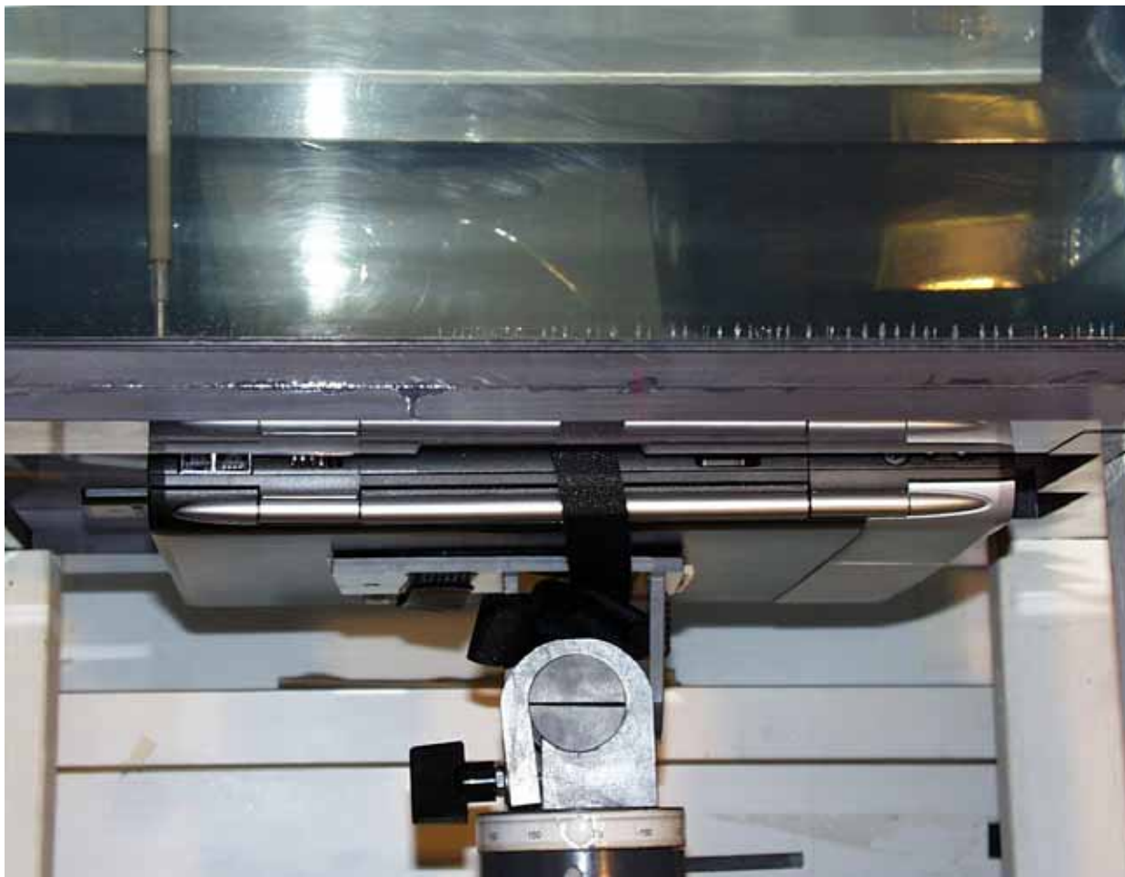
< Bottom of the host PC faced toward the phantom – 12 mm (Card-to-Bottom) >
