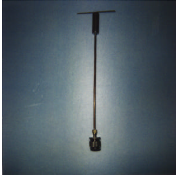
Fig. a. Photograph of the half-wave dipole at 1900 MHz used for system verification.
