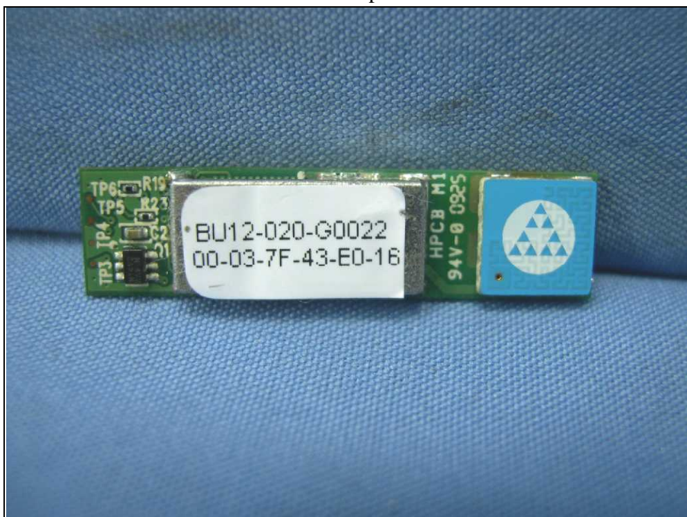
EUT with Chip antenna
