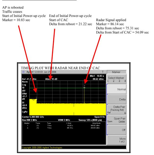
The radar signal is applied (86.14 - 10.83) = 75.31 seconds after reboot, which is 54.09 seconds after the completion of the initial power-up cycle.
