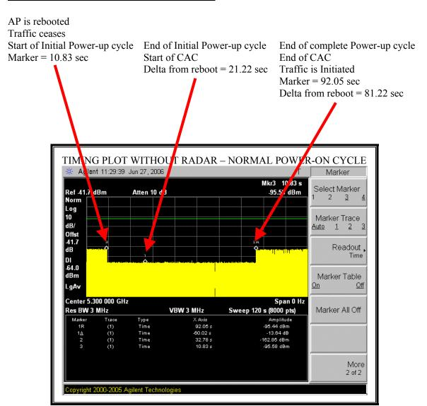
Note: The complete power-up cycle requires (92.05 - 10.83) = 81.22 seconds. The initial power-up cycle requires (81.22 - 60) = 21.22 seconds.
