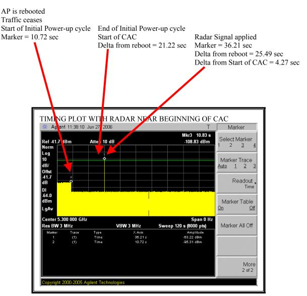
The radar signal is applied (36.21 - 10.72) = 25.49 seconds after reboot, which is 4.27 seconds after the completion of the initial power-up cycle.
