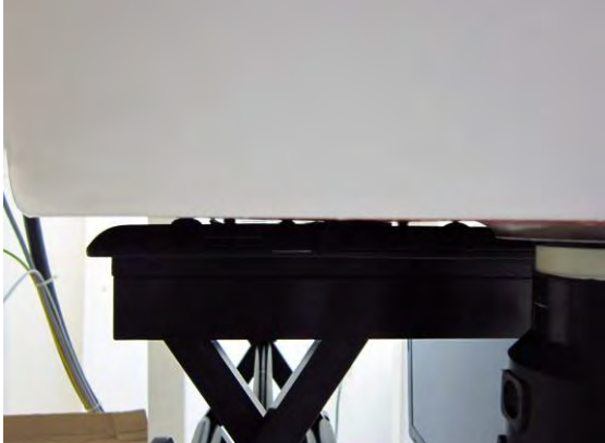
Fig.3 EUT Laptop mode to flat phantom
