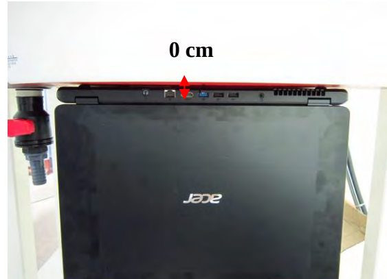
Fig.3 EUT Laptop mode to flat phantom
