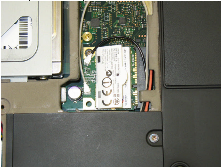
AR5B97 inside the Fujitsu TABLET Computer
