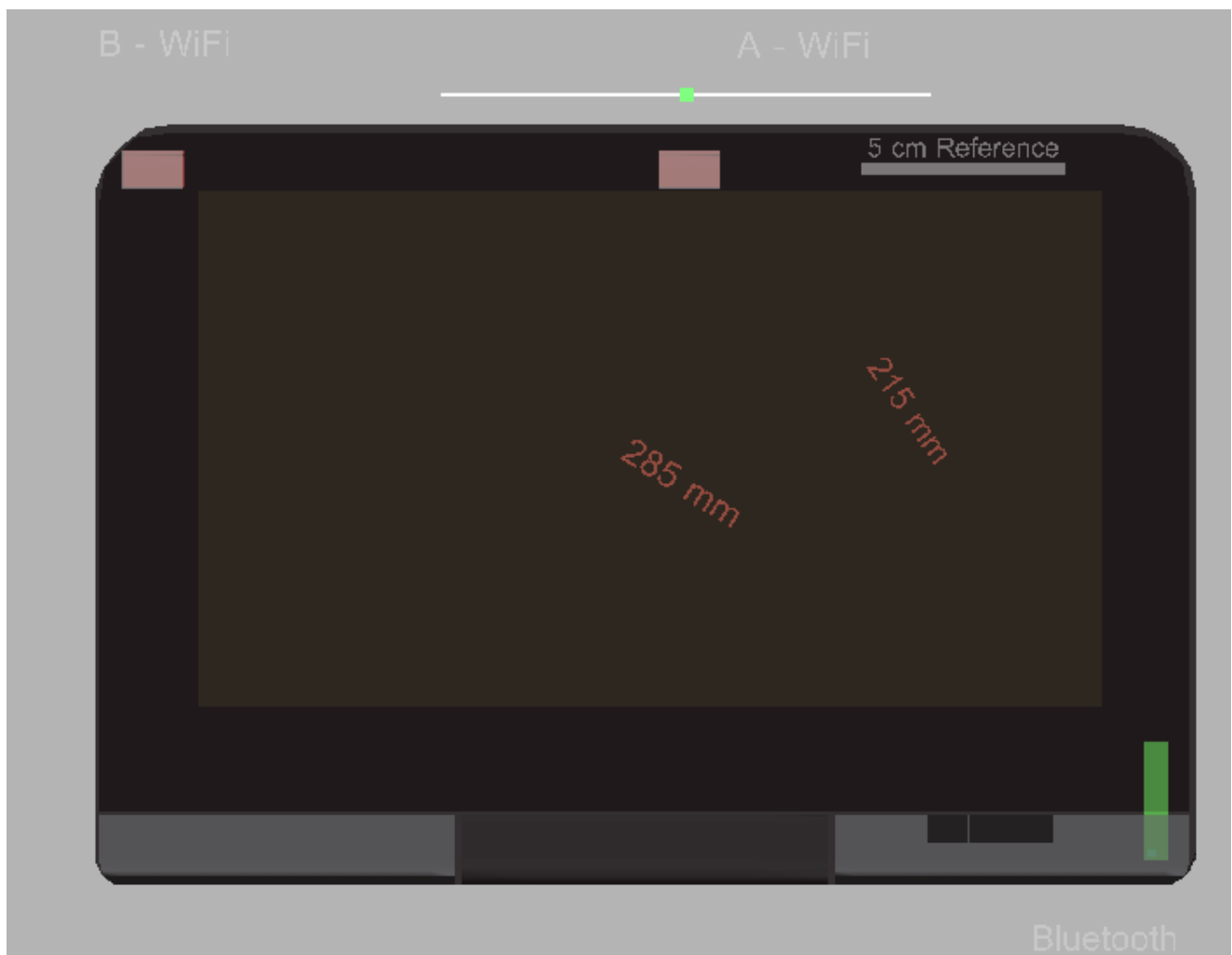
Diagram Showing distance between the Bluetooth and the WLAN antennas
