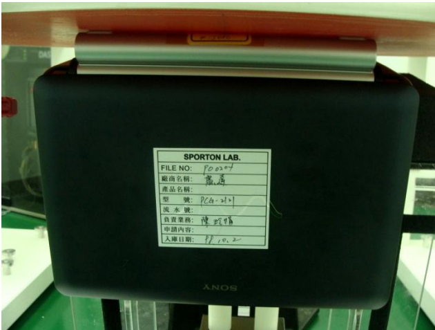
The Host with Battery 2 Bottom Touching Mode with 0 cm Air Gap – Front View
