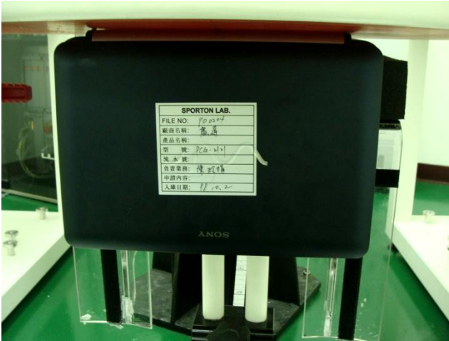
The Host with Battery 1 Bottom Touching Mode with 0 cm Air Gap – Front View
