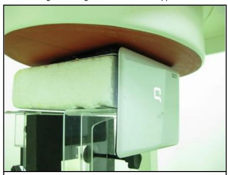
The bottom of the notebook contacts the bottom of the flat phantom with 0mm-separation distance.
