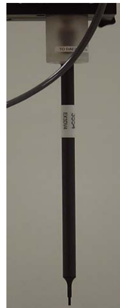
E-Field probe EX3DV4
