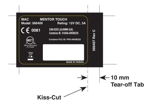
For dimensions and material specs, see engineering drawing. Add tear-off tab per this artwork.
