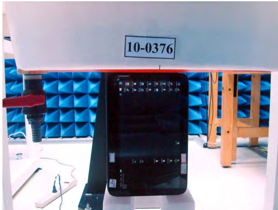
Figure 3. Body SAR Test Setup (Flat Section) Host Primary Portrait Close Body
