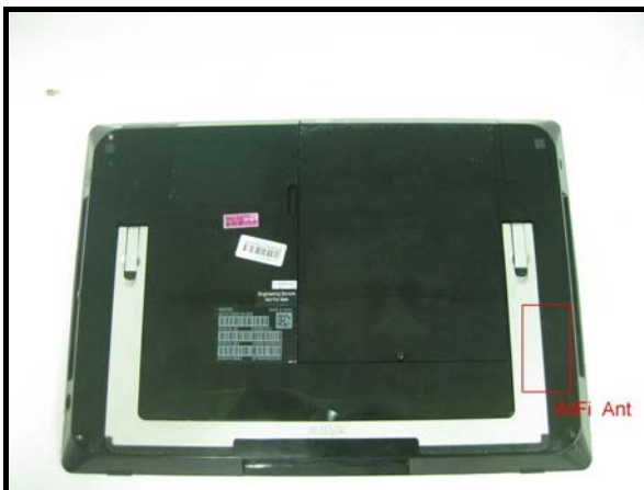
DESCRIPTION OF ANTENNA LOCATION
