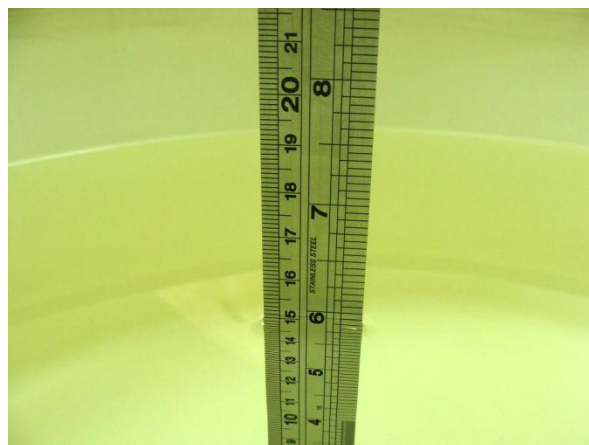
Fig 6.2 Photo of Liquid Height for Body SAR
