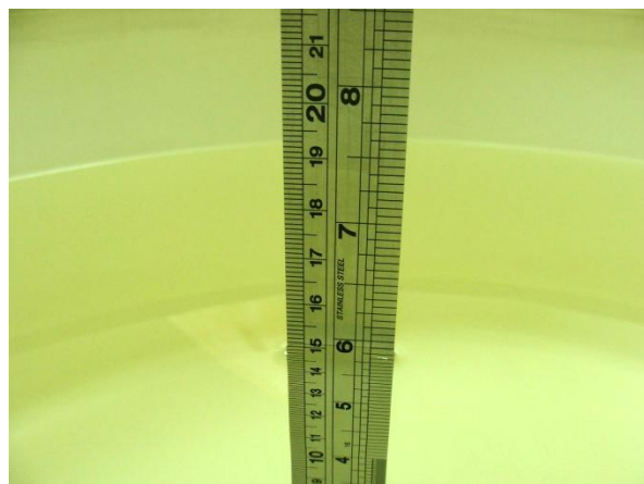
Fig 6.2 Photo of Liquid Height for Body SAR
