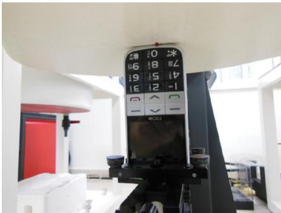
10mm Body-worn Bottom Side Setup Photo
