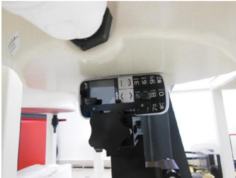
10mm Body-worn Right Side Setup Photo
