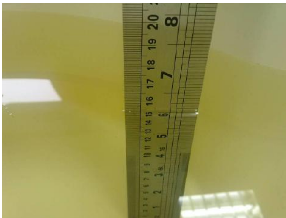
Photograph of the depth in the Body Phantom (835MHz)
