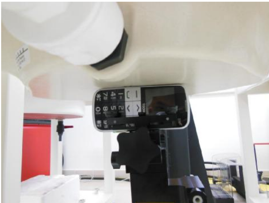
10mm Body-worn Left Side Setup Photo
