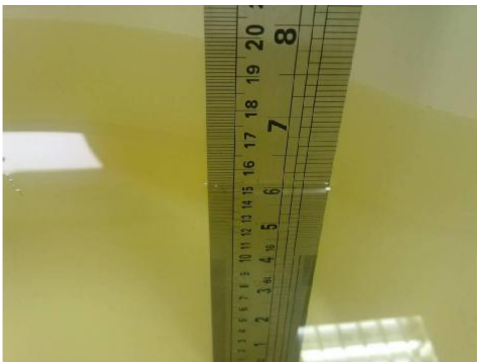
Photograph of the depth in the Body Phantom (1900MHz)
