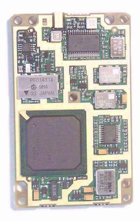
Networkcar Incorporated Wireless Modem, Model CR00R902M-2-O FCC ID: PP8CR00R902M-2-O
