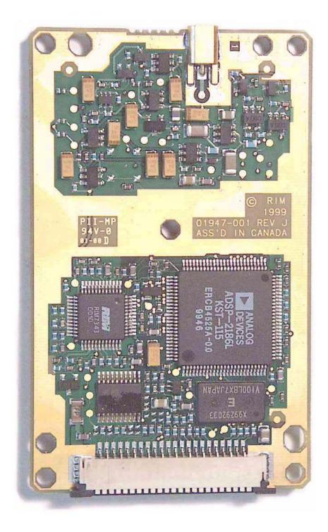
Networkcar Incorporated Wireless Modem, Model CR00R902M-2-O FCC ID: PP8CR00R902M-2-O
