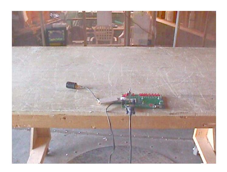
**EXHIBIT 9 - Test Setup Photos (Radiated Emissions Test Setup)**
