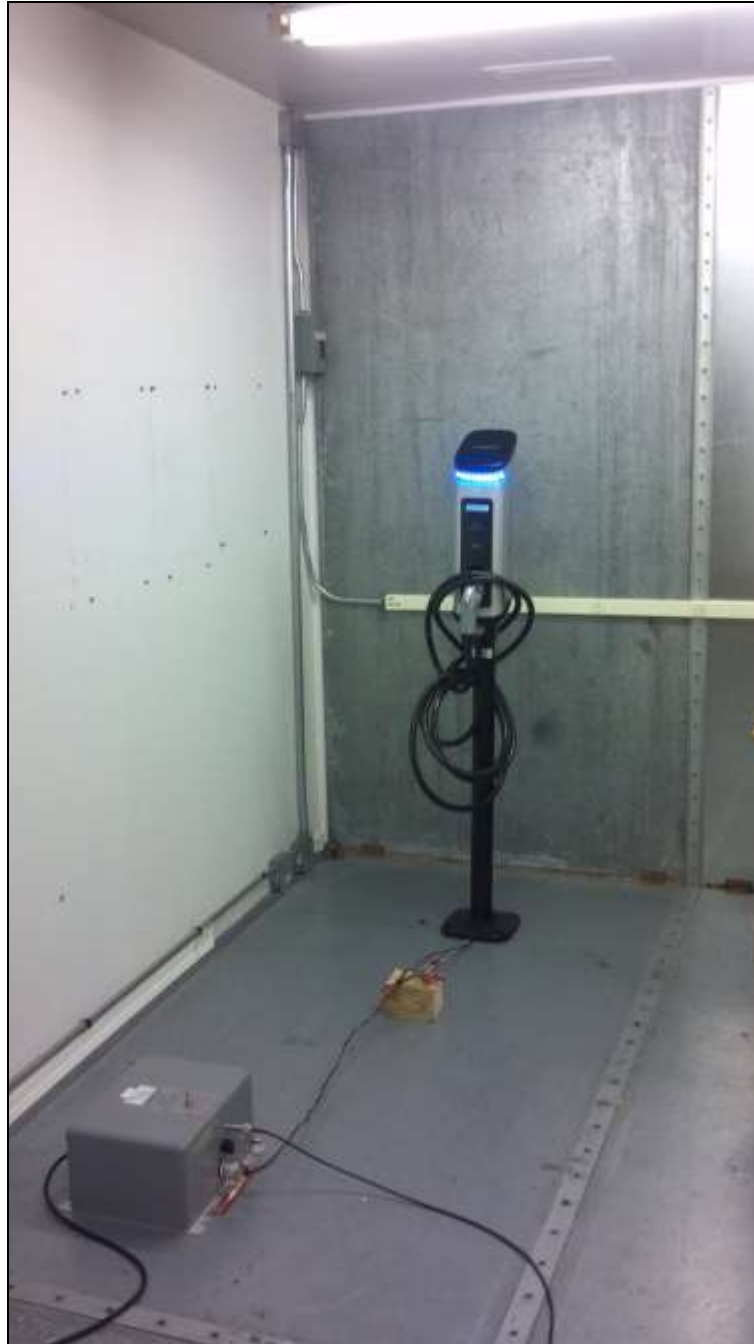
Photograph 1. Conducted Emissions, 15.207(a), Test Setup
