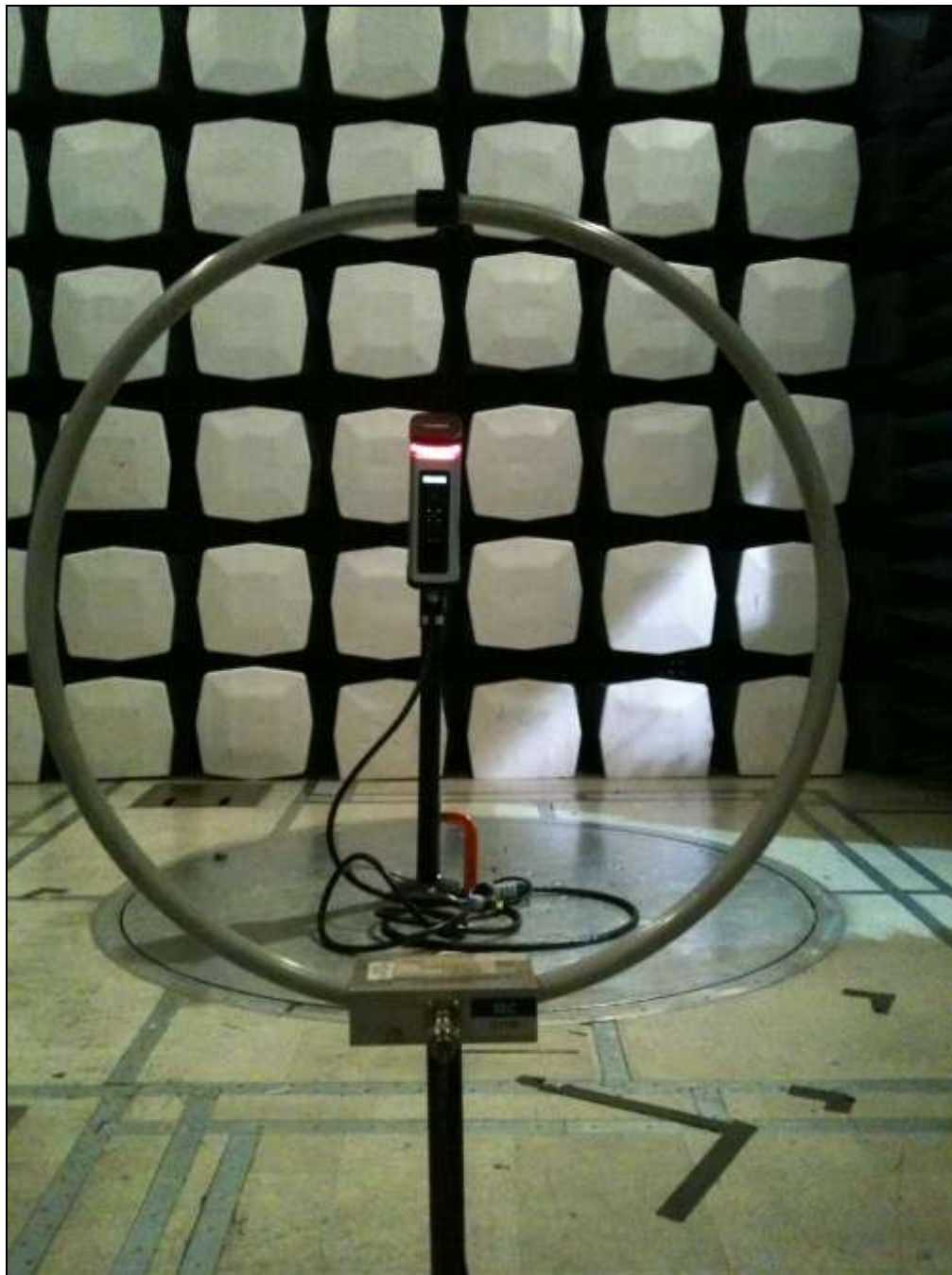
Photograph 2. Field Strength of Fundamental Emission, Test Setup
