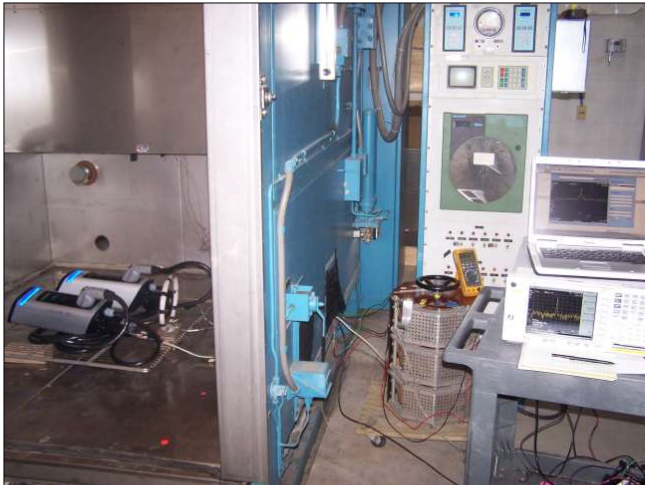
Photograph 4. Frequency Stability, Test Setup
