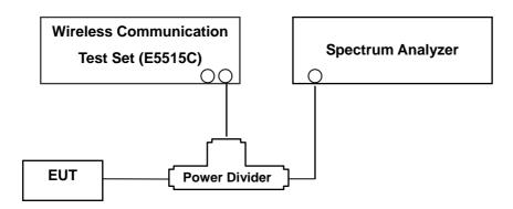
(Configuration of conducted Emission measurement)
