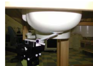
Fig. 18. Head SAR Test Setup
