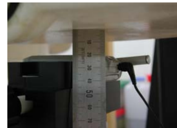
Fig. 21. Body SAR Test Setup with Holster
