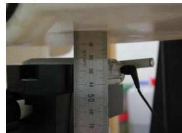
Fig. 20. Body SAR Test Setup with Holster
