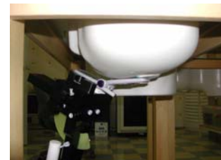
Fig. 14. Head SAR Test Setup
