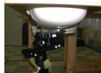
Fig. 18. Head SAR Test Setup
