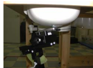
Fig. 19. Head SAR Test Setup
