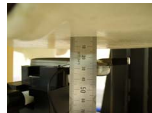
Fig. 20. Body SAR Test Setup with Holster
