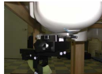
Fig. 15. Head SAR Test Setup
