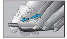
NOTE: If the battery is not correctly placed in the battery compartment, the handset will not turn on and/or the battery may detach during use.
