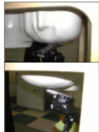
Fig. 17. Head SAR Test Setup
