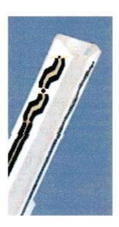
Figure 5. ET3DV6 E-field Probe
