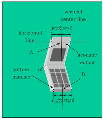
Figure 7. Device Test Position
