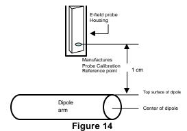
Separation Distance from Dipole to Field Probe
