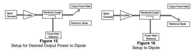
Using this setup configuration, the signal generator was adjusted for the desired output power (100mW) at a specified frequency. The reference power from the coupled port of the directional coupler is recorded. Next, the output cable is connected to the reference dipole, as shown in Figure 16.
