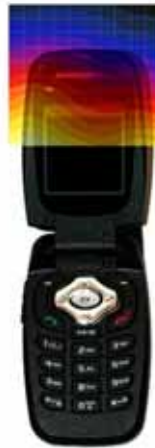
Figure 28 Sample H-field Scan Overlay
