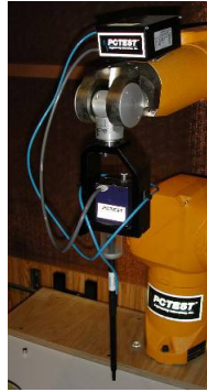
Figure 6 SPEAG Robotic System
