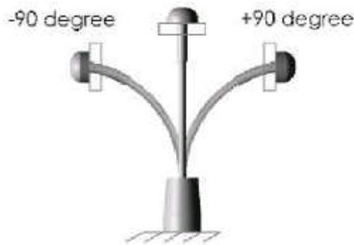
Figure 3-4: Whip bending test
