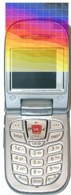
Figure 28 Sample H-field Scan Overlay
