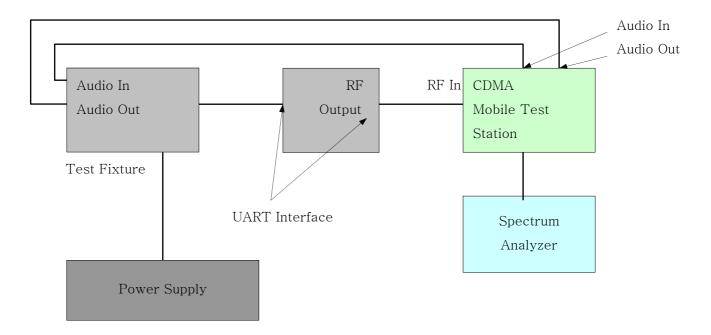
UART Interface: The UART Interface has a serial communication link and RF Interface port that can be used to test, debug or upgrade the phone's functions and characteristics.
