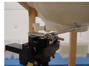
Fig. 18. Head SAR Test Setup
