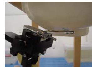
Fig. 15. Head SAR Test Setup
