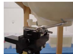
Fig. 19. Head SAR Test Setup
