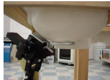
Fig. 16. Head SAR Test Setup
