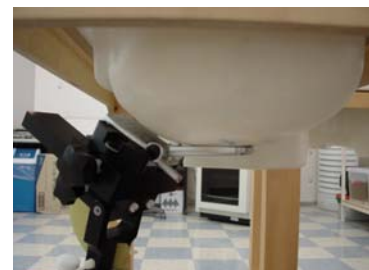
Fig. 15. Head SAR Test Setup
