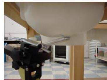
Fig. 17. Head SAR Test Setup
