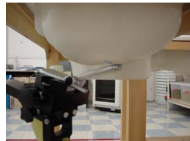
Fig. 18. Head SAR Test Setup
