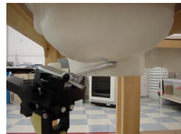
Fig. 19. Head SAR Test Setup
