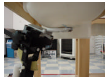
Fig. 14. Head SAR Test Setup
