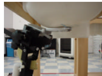
Fig. 16. Head SAR Test Setup
