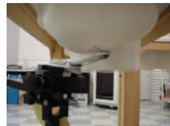
Fig. 17. Head SAR Test Setup
