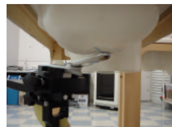
Fig. 19. Head SAR Test Setup
