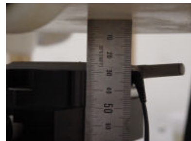
Fig. 22. Body SAR Test Setup with Holster
