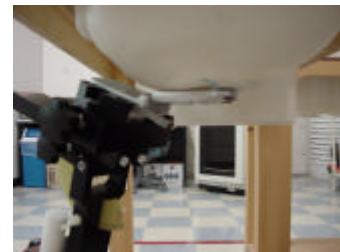
Fig. 15. Head SAR Test Setup
