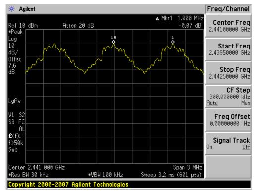
Test Plot 20 dB bandwidth (Low CH)
