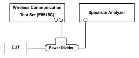
(Configuration of conducted Emission measurement)
