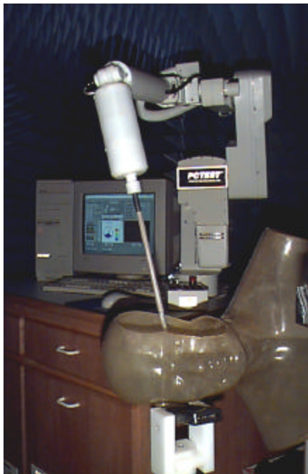
Figure 5. Photograph of the Probe and the Phantom
