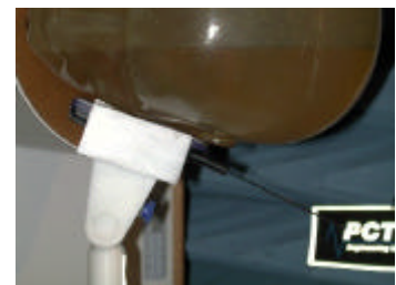
Figure 14. Head SAR Test Setup
