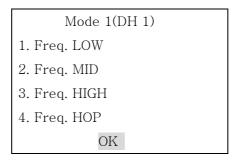
f. Selecting "Freq. LOW" item will transmit DH 1 packet in low cannel. You can see screen below. You will select [OK] soft key to exit this menu.
