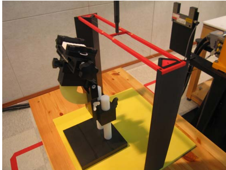
Figure 2. HAC Phantom & Device Holder
