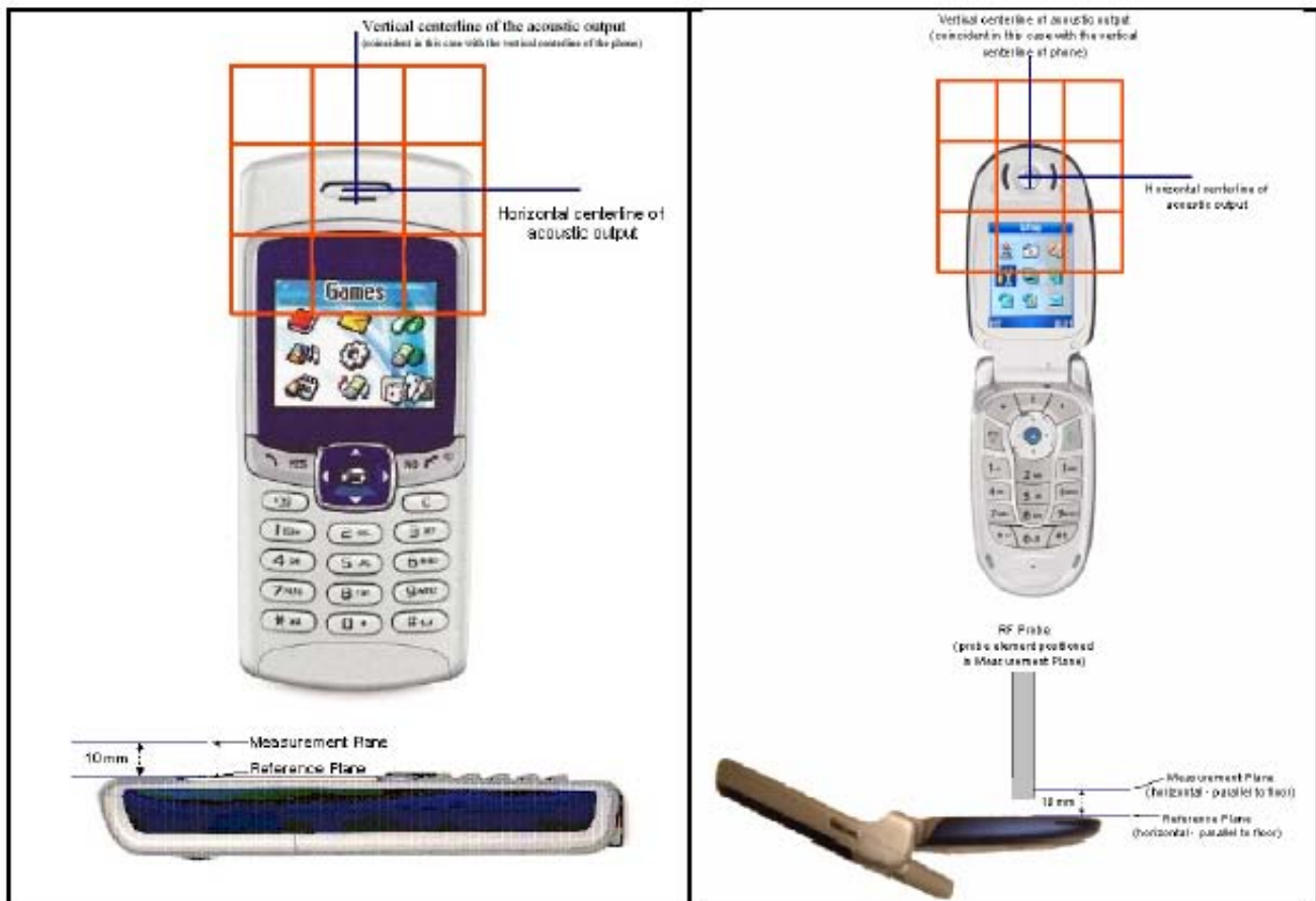
Figure 3. WD reference and plane for RF emission measurements
