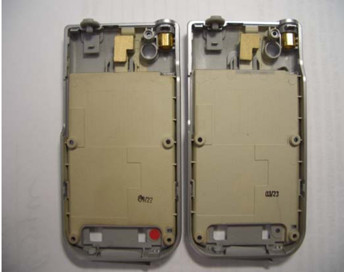
4 LCD Module : Vender change ( ODT -> HYeLCD ). Before ( Left ) ----> After ( Right )
