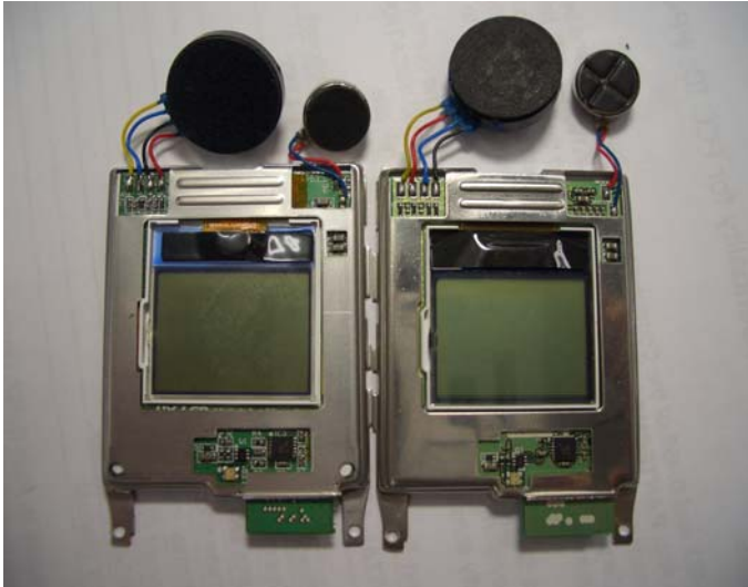
5 LCD FPCB : Vender change ( Daeduck GDS -> BHFlex ). Before ( Left ) ----> After ( Right )
