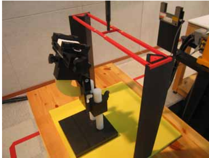
Figure 2. HAC Phantom & Device Holder
