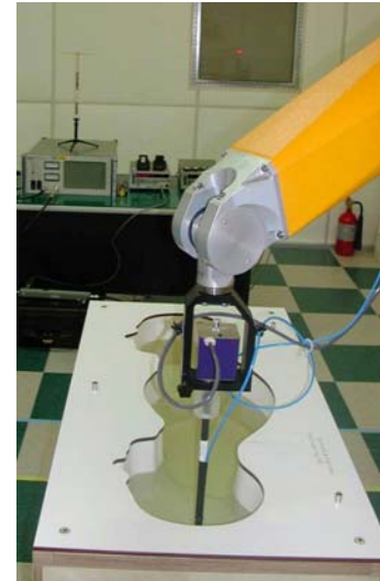
Figure 4. Photograph of the probe and the Phantom
