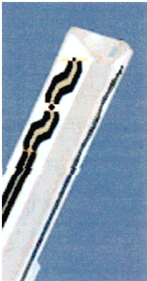
Figure 5. ET3DV6 E-field Probe
