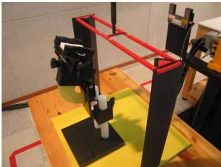
Figure 2. HAC Phantom & Device Holder
